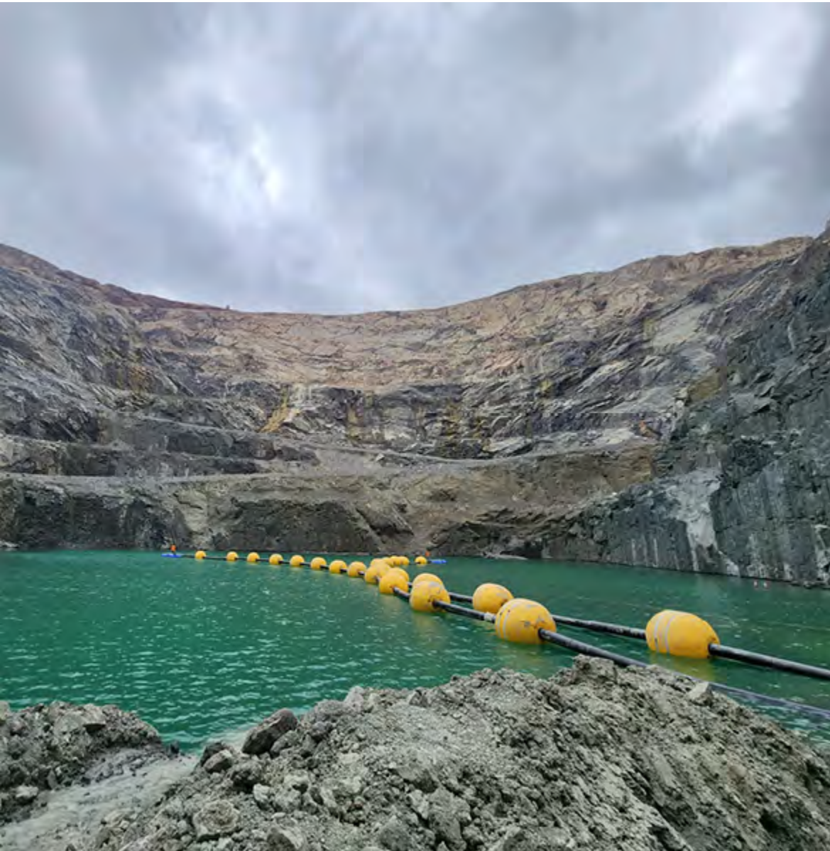
Venetia storm water management - K03 dewatering infrastructure.
