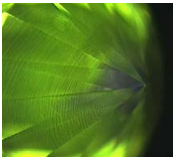
DiamondView™ image of a CVD synthetic diamond that has been heat treated after growth
