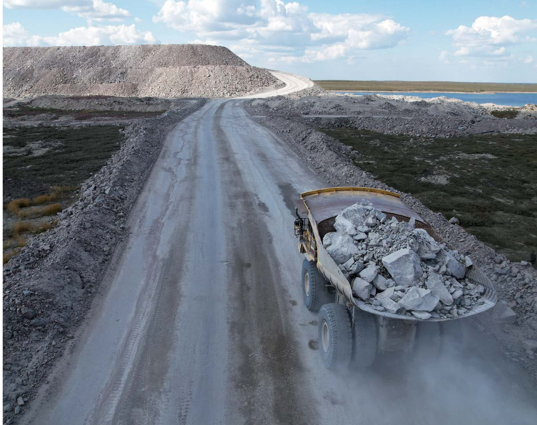
A haul truck carries a load of mine rock to the west mine rock pile at Gahcho Kué mine.
